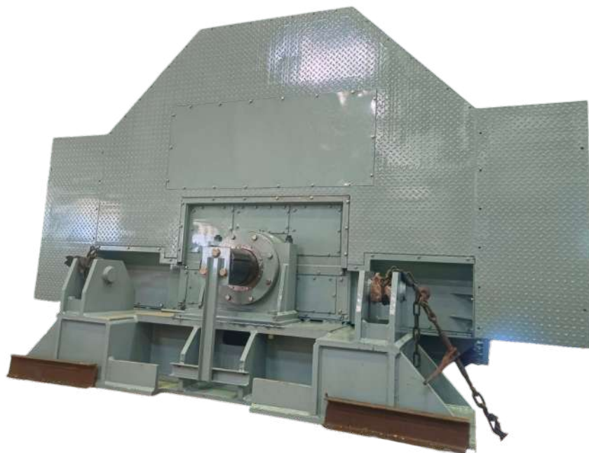
2x750kW, 300V, 200/300 RPM KWDC3106, Twin armature Rolling mill high inertia load application.
